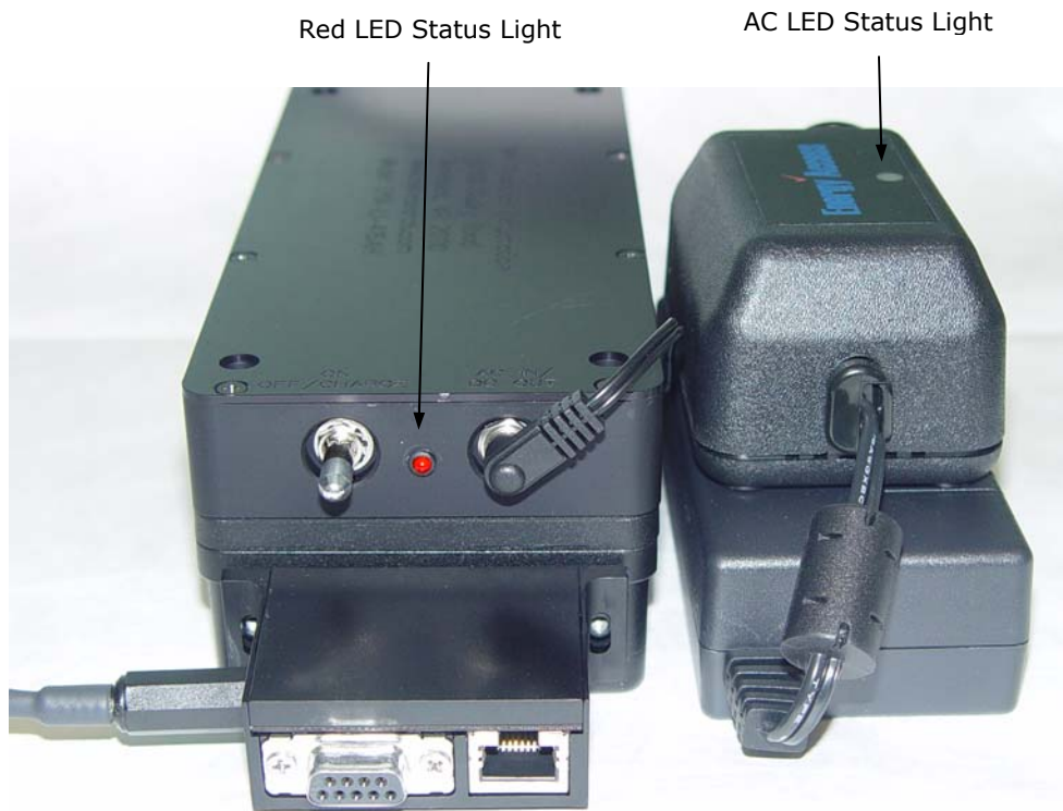
Figure 3. Battery pack being charged by the AC adapter.
