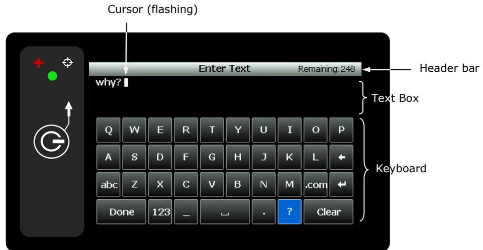
The keyboards are used to enter text inside the text box. The recommended hand-position is shown in the figure below utilizing two thumbs to tap the keyboard. While entering text, the position of the cursor in the text box is shown as a flashing white block. The block turns red when the maximum limit is reached (Remaining: 0). An alert will sound when the maximum number of characters is exceeded and additional text is entered.
