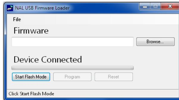
2. With a USB cable attached to a computer and the device, press the "Start Flash Mode" button.
