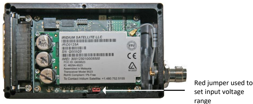
Figure 2: Power Input Setting for the A3LA-RM
