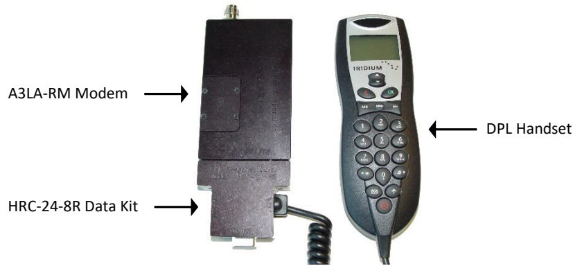
Figure 2: A3LA-RM Connected to a DPL Handset via the HRC-24-8R
