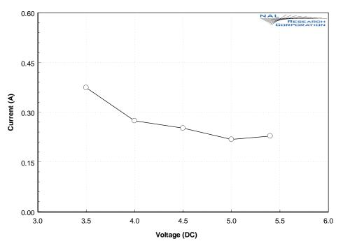
Figure 5: Average Current Drawn During an SMS Transmission
