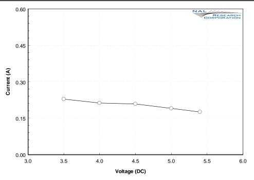
Figure 4: Average Current Drawn During an SBD Transmission
