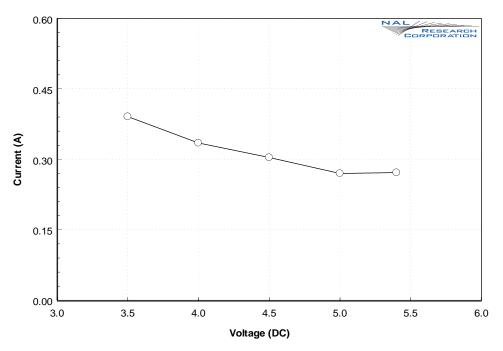
Figure 3: Average Current Drawn During a Data Switch Call
