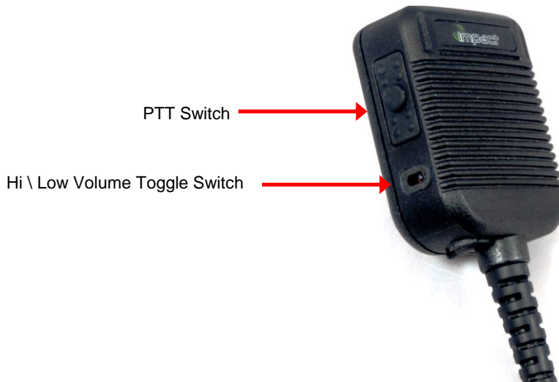
Figure 154: Speaker-Microphone PTT Switch and Hi/Low Toggle Switch
