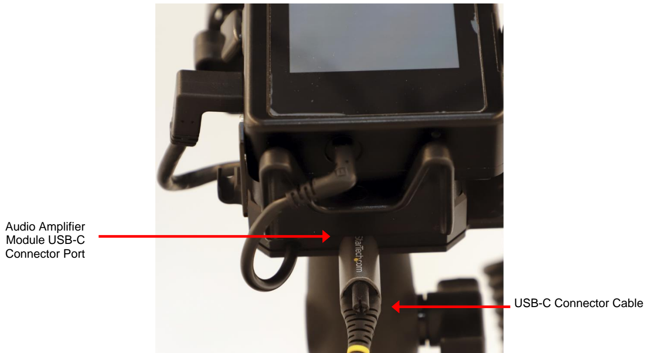
Figure 152: Power Connection to Audio Box
