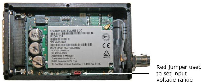
Figure 2. Power Input Setting for the A3LA-RM.
