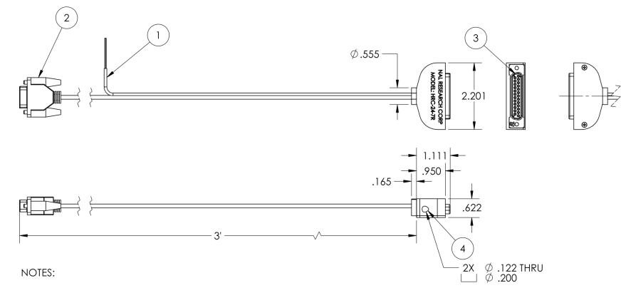
5-32 VDC INPUT (+) RED (GND) BLACK SERIAL DATA CONNECTOR (FEMALE DB-9) DATA/POWER CONNECTION TO MODEM (FEMALE DB-25) MOUNTING HOLES TO MODEM. 2X 4-40 SOCKETHEAD SCREWS PROVIDED
