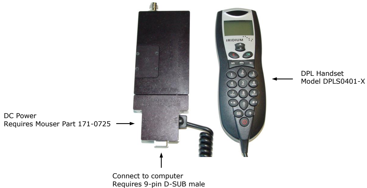
Figure 1. A3LA-R Connected to a DPL handset and HRC-24-8R data Kit.
