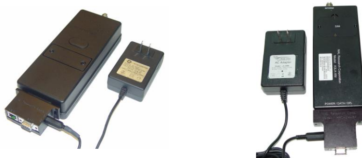
Figure 2. Model LA-3098 connected to an A3LA-D/-XM via the HRC-24-8/8X DB25 data kits.
