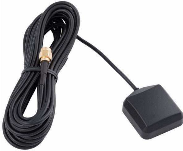
Model SAF5270-G is a miniature active GPS antenna designed to operate with the NAL Research satellite modems and trackers. It provides coverage at 1575.42 MHz (L1). The SAF5270G is water-resistant and has a magnetic mounting for quick, convenient placement on or inside vehicles.
