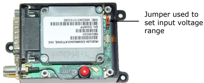
Figure 3: Power Input Setting for the 9602-LP
