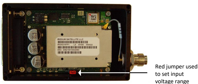
Figure 3: Power Input Setting for the A3LA-RG
