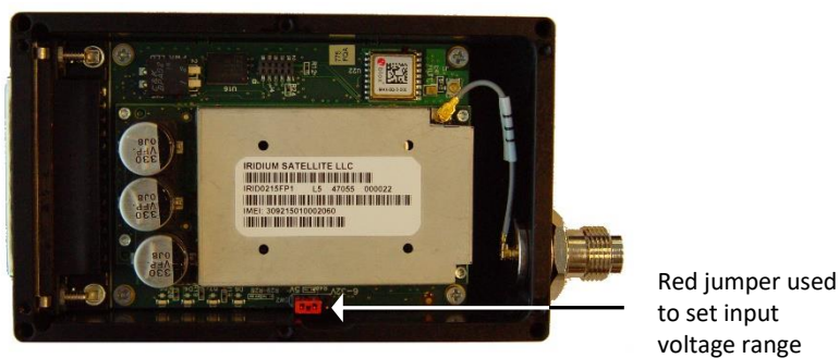
Figure 3: Power Input Setting for the A3LA-RG
