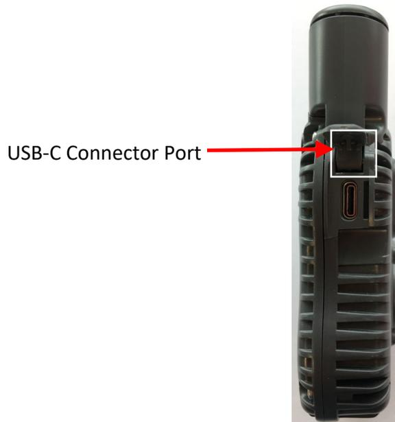
*Figure 5: USB Connector Port*
