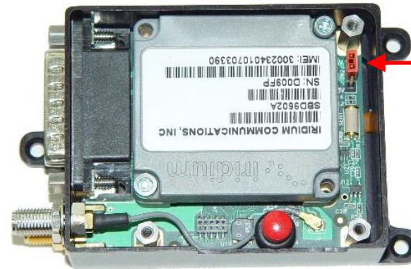
Jumper used to set input voltage range
