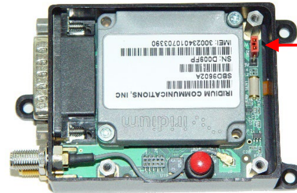
Jumper used to set input voltage range
