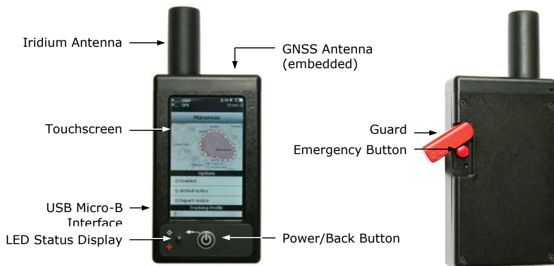
Figure 1: SHOUT ts Exterior Components
