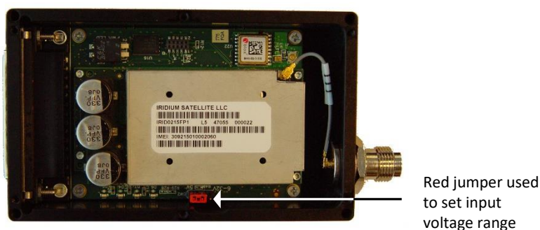
Figure 3: Power Input Setting for the A3LA-RG
